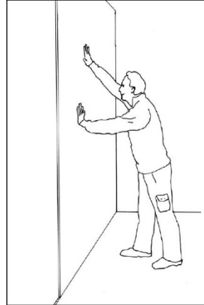
Lock panel in place by applying pressure with the palm of the hand
